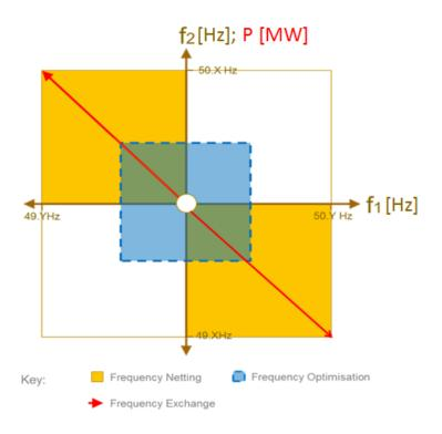
Figure 1: Illustration of the different frequency coupling classes and how they relate to the frequencies of the synchronous areas (showing two synchronous areas only). For frequency exchange, the x-axis (f1 [Hz]) relates to the frequency of the receiving SA, whereas the y-axis (P[MW]) relates to the power shifted from providing to receiving SA.
